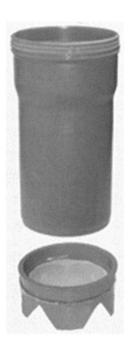
Figure. 1. The feather lice strainer is made of a 20 cm PVC waste pipe and a 6 cm high socket made from a pipe coupling, and equipped with a 400 micron plankton net. The internal diameterof the pipe is 10 cm. The pipe coupling has been cut so the wider part is 2 cm high, sawn through below and glued together with the plankton net in between. As the water must flow easily from the strainer the socket has been sawn so that it stands on four legs.
