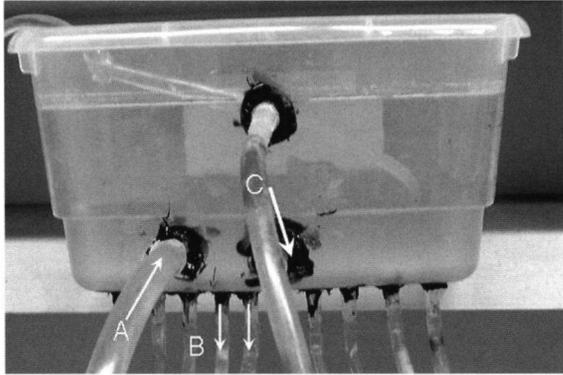
Fig. 4. Head tank which contains filtered water. A. indicates filtered water from the filter box (Fig. 3). B. indicates water fed by gravity to the housing chamber boxes (Fig. 2, 3). C. indicates overflow water back to the filter box (Fig. 3).
