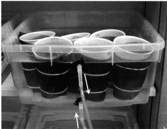
Fig. 2. Translucent box used to contain housing chambers for libellulid larvae. The polyethylene box is 38×38×16.5 cm and can hold up to 10 housing chambers (Fig. 1). Arrows indicate flow of water through plastic tubing.
