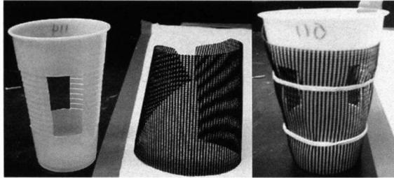
Fig. 1. Housing chamber for libellulid larvae. Chamber is made from a 480 ml (16 oz) plastic drinking cup with 3×5 cm windows. The chamber is surrounded by nylon window screen to allow water to flow but retain the larvae. One chamber holds 1-3 larvae.
