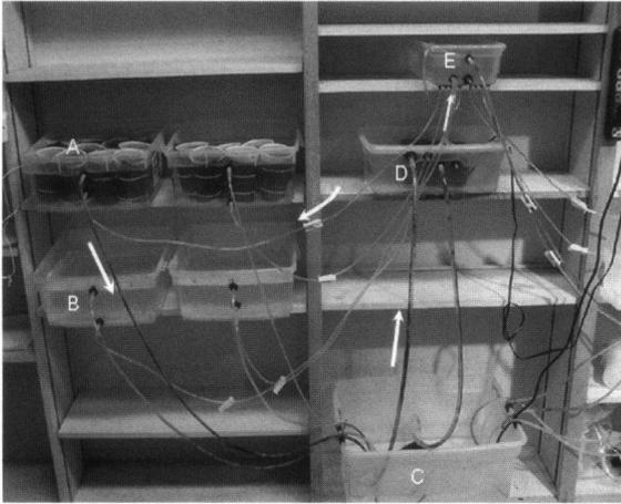
Fig. 3. Recirculating system for maintaining libellulid larvae. A. is an individual housing chamber (Fig. 1). B. is the box which contains several housing chambers (Fig. 2). C. is the large waste water container, which pumps water up to D. the filter box. From the filter box, clean water is pumped to E. head tank (Fig. 4), which feeds to the housing chamber box B. Arrows indicate flow of water through plastic tubing.
